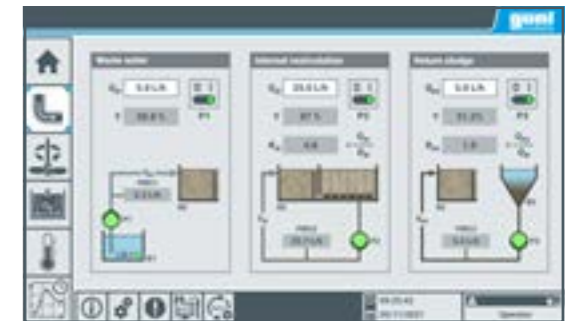
Touch screen: operation of the pumps
