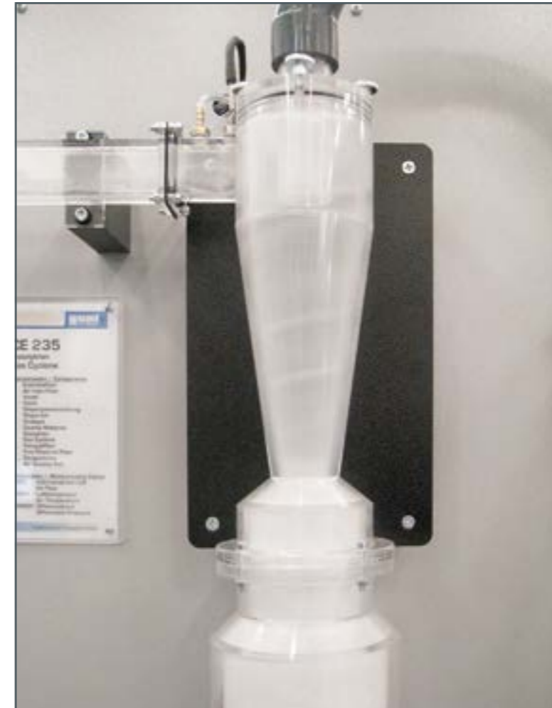
Separation of respirable crystalline silica in the gas cyclone during a test run in our laboratory. You can see the spiral motion of the particles which is characteristic of cyclones.
