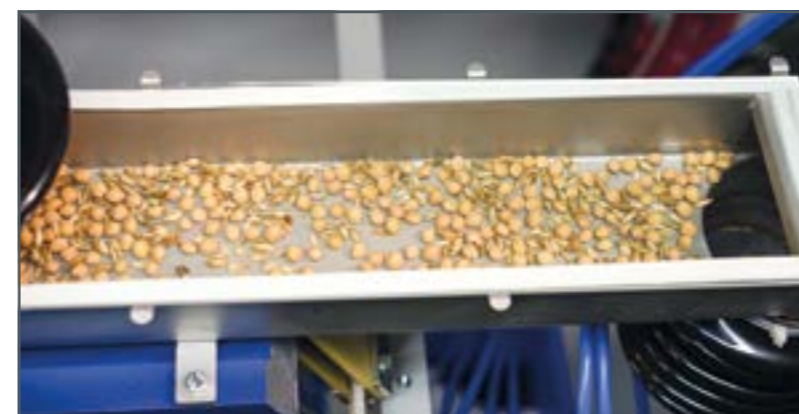
CE 275 during a trial run: The vibrating trough evenly conveys the mixture of spelt husks and cherry stones to be separated from to the zigzag sifter.
