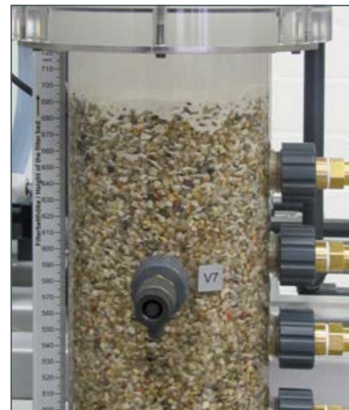
Transparent filter tube to observe the increased loading of the filter bed
