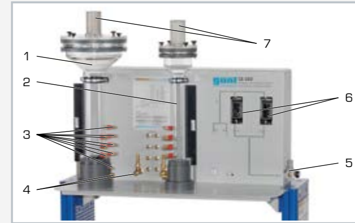
1 column K1 with \varnothing 100mm, 2 column K2 with \varnothing 50mm, 3 differential pressure measuring points of K1, 4 gas supply for K1, 5 gas supply to the trainer, 6 flow measurement for 2 measuring ranges, 7 air filter
