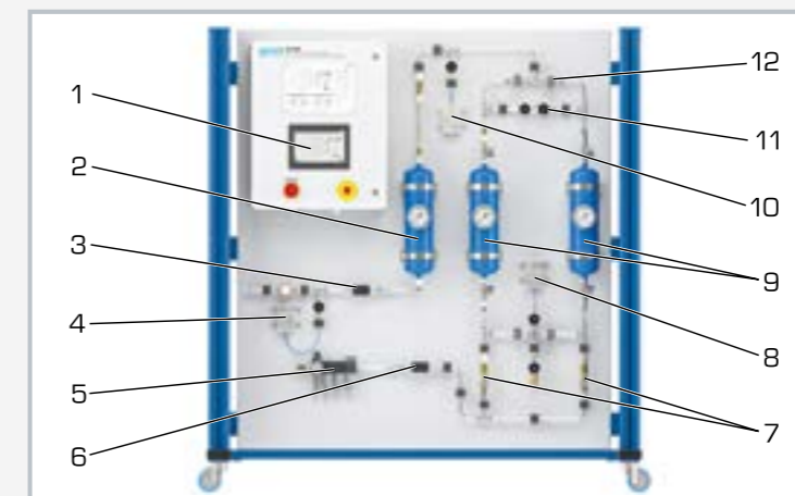
1 PLC with touch screen, 2 storage tank, 3 sensors for temperature, pressure and flow rate in the product gas, 4 sensor for oxygen concentration in the product gas, 5 maintenance unit and pressure controller, 6 sensors for temperature, pressure and flow rate in the compressed air, 7 and 12 solenoid valves for pressure swing and column change-over, 8 sensor for oxygen concentration in the exhaust gas, 9 columns, 10 sensor for oxygen concentration in the breakthrough measurement, 11 partial purge gas flow adjustment
