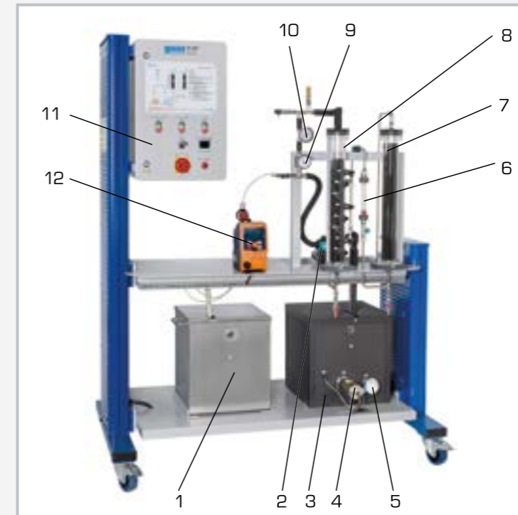
1 adsorbate solution tank, 2 circulation pump, 3 treated water tank, 4 heater, 5 temperature sensor, 6 flow meter, 7 safety adsorber, 8 adsorber, 9 thermometer, 10 manometer, 11 switch cabinet, 12 metering pump
