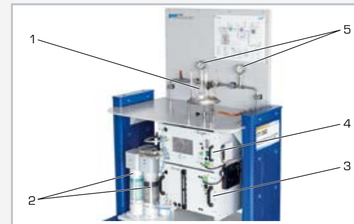
1 gas burner, 2 raw water purification, 3 tank for purified water, 4 AEM electrolyser with tank for potassium hydroxide, 5 manometers for hydrogen pressure
