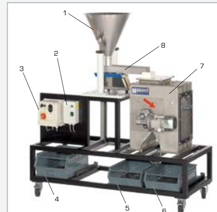
1 feed hopper with height adjuster, 2 vibrating trough controls, 3 magnetic separator controls, 4 solid compound tank, 5 magnetic materials tank, 6 non-magnetic materials tank, 7 magnetic separator, 8 vibrating trough
