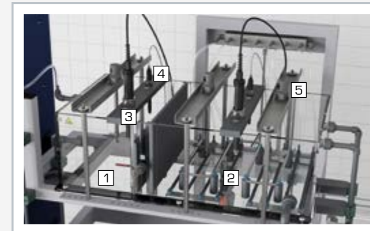
Aeration tank: 1 denitrification zone (non-aerated), 2 nitrification zone (aerated), 3 oxygen sensor, 4 pH value sensor, 5 stirring machine
