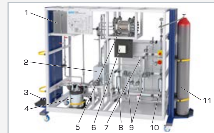
1 storage tank with distilled water, 2 tank with purified water, 3 holder for N 2 gas cylinder, 4 ion exchanger, 5 PEM electrolyser, 6 gas cooling, 7 filter, 8 condensate tank, 9 adsorption dryer installed in parallel, 10 H 2 buffer tank, 11 H 2 gas cylinder
