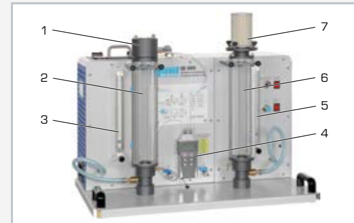
1 water overflow, 2 tank for water, 3 rotameter for water, 4 hand-held measuring unit pressure loss, 5 rotameter for air, 6 tank for air, 7 filter
