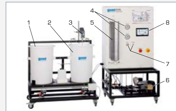
1 rinsing water tank (distilled water), 2 raw water tank (salt solution), 3 stirring machine, 4 manometer, 5 spiral wound membrane module, 6 pump with motor, 7 valves, 8 PLC with touch screen
