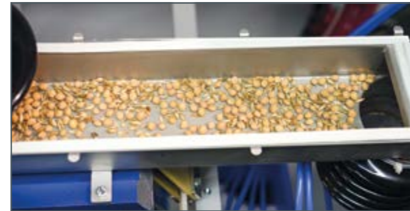
CE 275 during a trial run: The vibrating trough evenly conveys the mixture of spelt husks and cherry stones to be separated from to the zigzag sifter.
