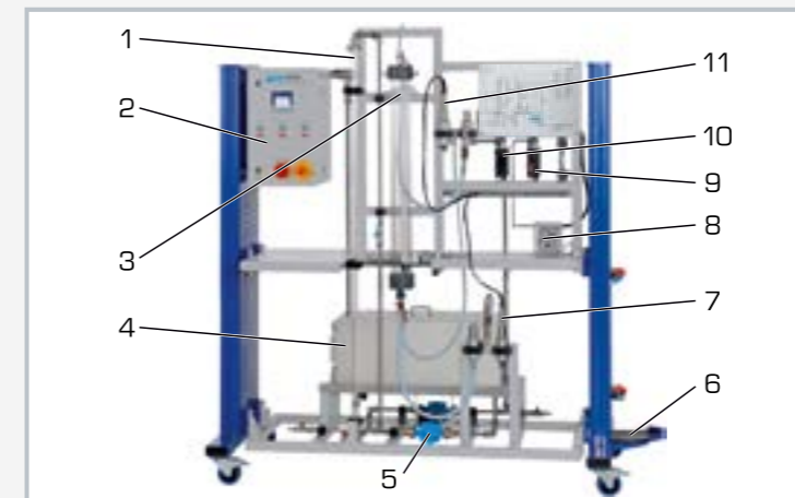
1 desorption column, 2 switch cabinet, 3 absorption column, 4 tank, 5 pump, 6 mounting for pressurised gas cylinder, 7 oxygen and temperature sensor downstream of absorption, 8 compressor, 9 flow meter (air), 10 flow meter (water), 11 oxygen and temperature sensor upstream of absorption
