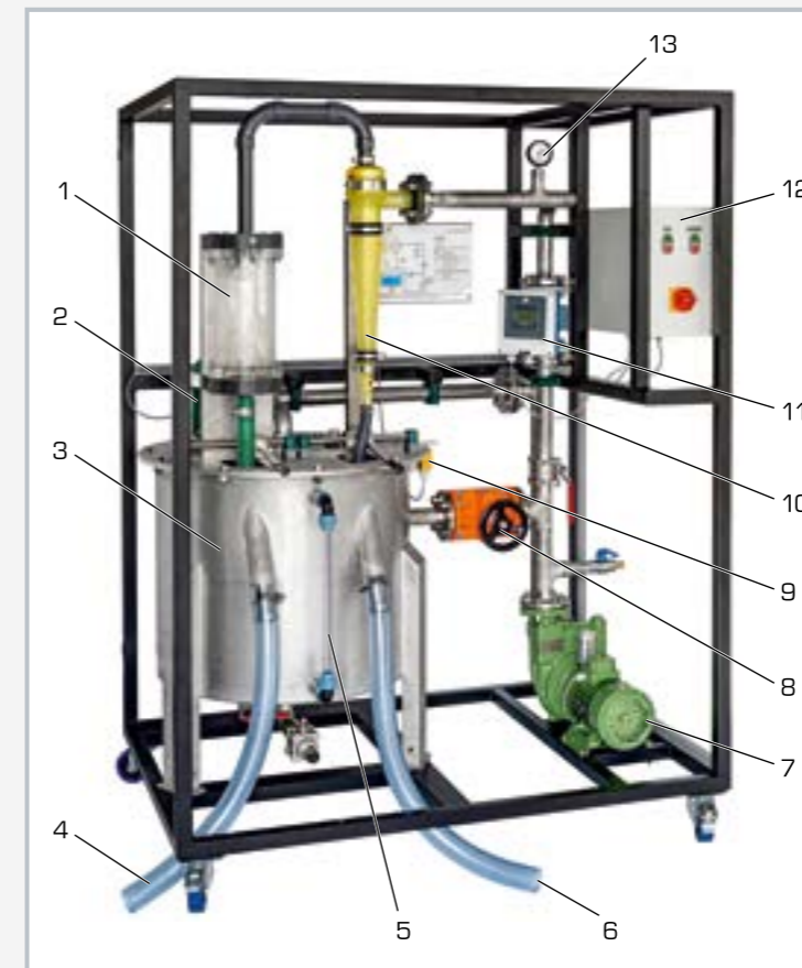
1 tank for observation of overflow, 2 stirring machine, 3 stirred tank, 4 overflow sampling point, 5 level indicator, 6 underflow sampling point, 7 pump, 8 valve in bypass, 9 safety switch, 10 hydrocyclone, 11 flow meter, 12 switch box, 13 manometer
