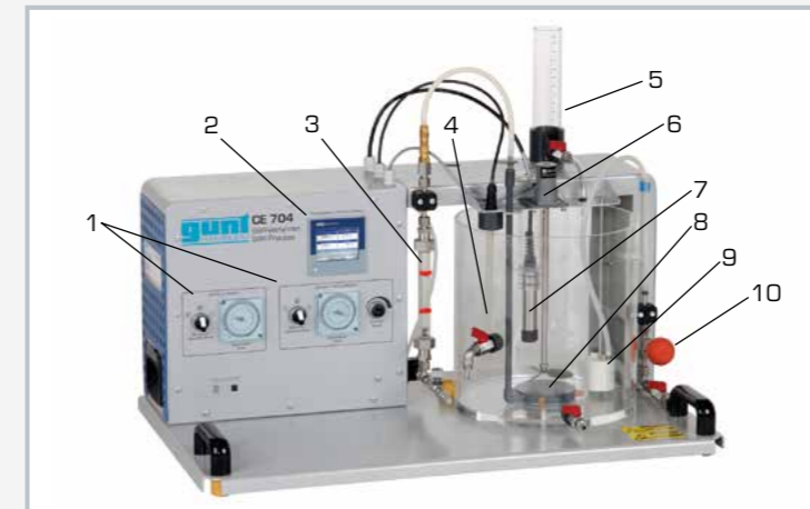
1 control elements for the compressor and for the stirring machine, 2 process controller, 3 flow meter (air), 4 pH value sensor, 5 metering device, 6 stirring machine, 7 oxygen sensor, 8 aeration device, 9 float for clear water extraction, 10 suction bulb for clear water
