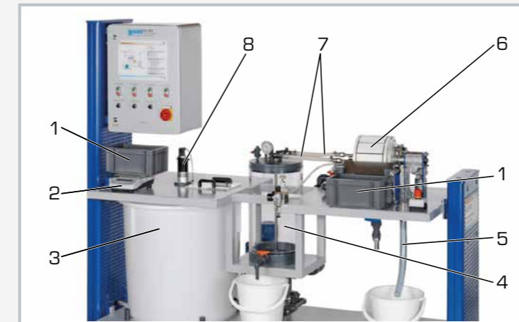
1 filter cake collector tank, 2 balance, 3 suspension storage tank, 4 filtrate vacuum tank, 5 overflow/outlet, 6 drum cell filter, 7 vacuum supply, 8 stirrer
