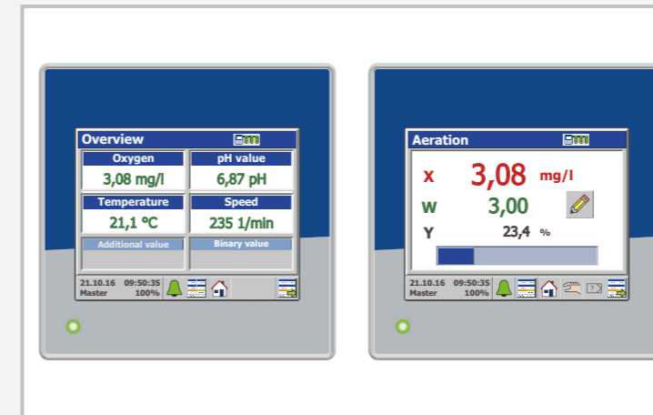
Digital process controller display of process variables (left), user interface for controlling oxygen concentration (right)
