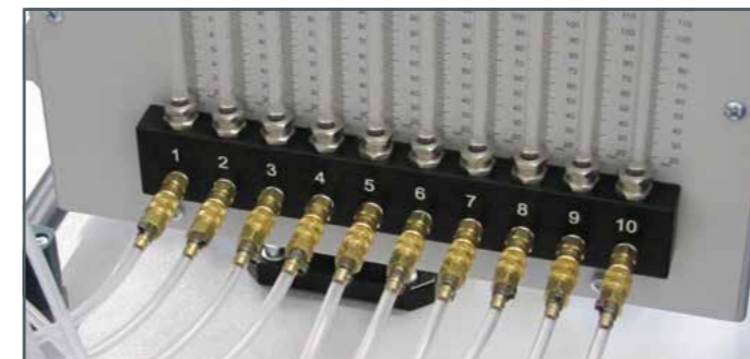
Connections on the manometer panel for measuring the pressure in the filter bed
