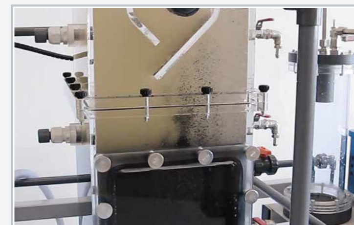
UASB reactor during experimental operation
