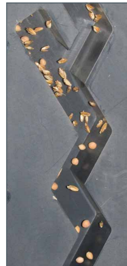
CE 275 during a trial run: The vibrating trough evenly conveys the mixture of spelt husks and cherry stones to be separated from to the zigzag sifter.
