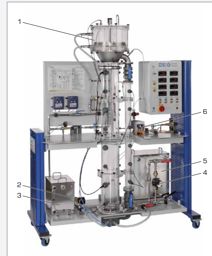
1 airlift reactor with external circulation, 2 feed pump, 3 feed tank, 4 circulating pump, 5 storage tank, 6 metering pump
