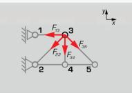
Method of joints: freeing the bar forces at node 3
