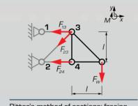
Ritter's method of sections: freeing the bar forces at nodes 3 and 4
