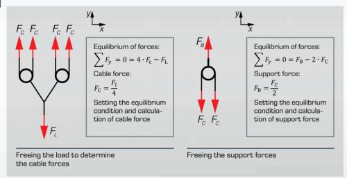
Checking the calculation: comparison of results with the measured values on suspension cable/supports and the results from the GUNT software
