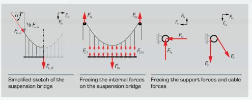
Calculation of external and internal forces with additional loading by single load, line load or moving load
