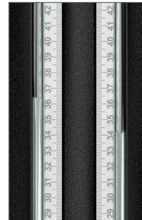
The tube manometer enables low pressure losses to be determined with a high degree of accuracy.
