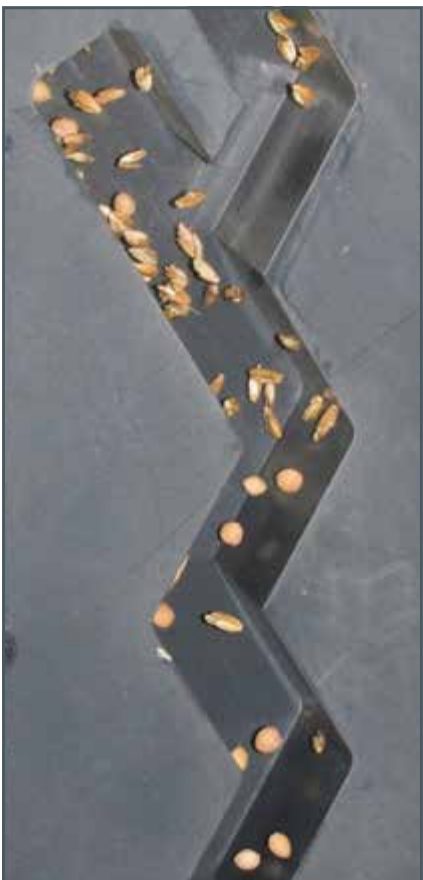
In the zigzag channel, the separation of the mixture can clearly be observed.
