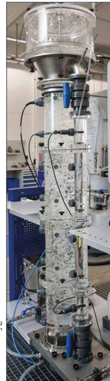
Airlift reactor during a test run
