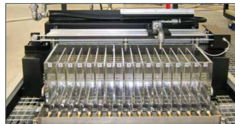
The measuring chambers are filled successively in a time controlled manner.
