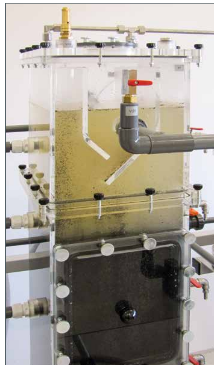
CE 702's UASB reactor during a successful trial run in our laboratory
