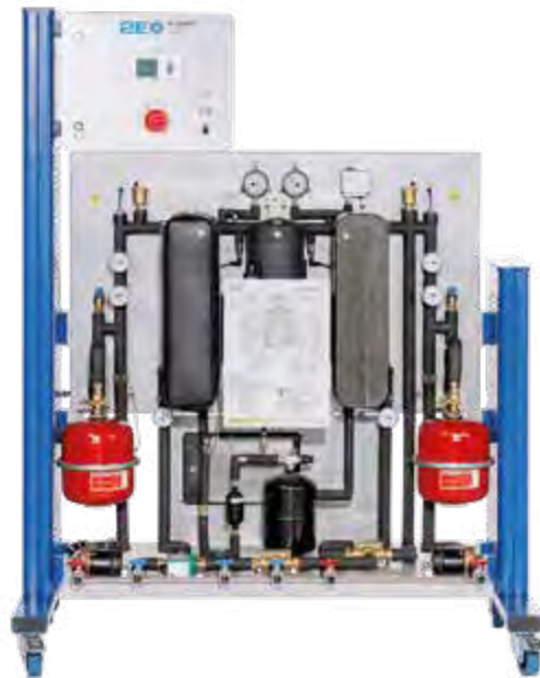
HL 320.01 Heat pump Heat pump for operation with different sources, operating the heating controller via web browser
