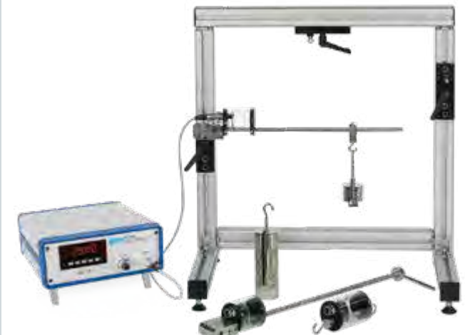
FL 100 Strain gauge training system
