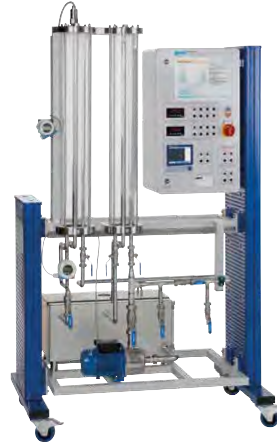
HM 500 Flow meter trainer Comparison and calibration of different flow meters
