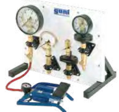
HM 700.16 Cutaway models: pressure gauges
