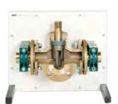
HM 700.12 Cutaway model: three-way plug valve
