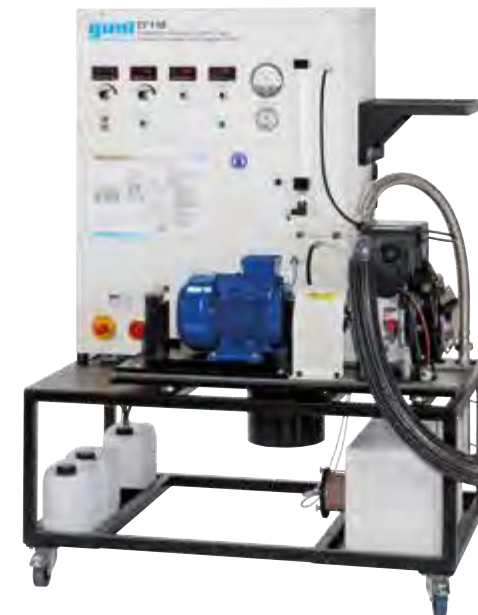
CT 100.22 Four-stroke diesel engine for CT 110
