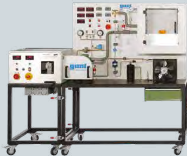
Compression refrigeration system ET 165 with drive unit HM 365
