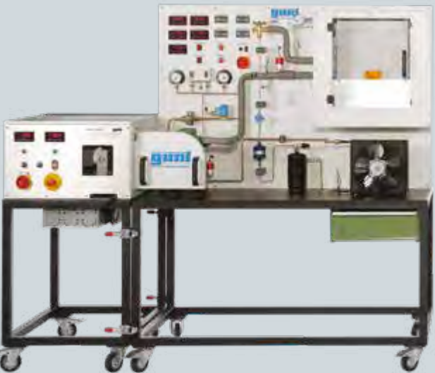
Compression refrigeration system ET 165 with drive unit HM 365
