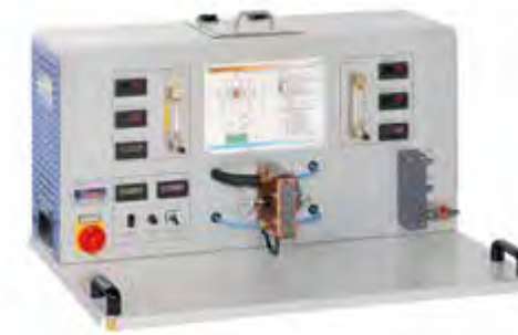
ET 360 Refrigeration circuit with propane
