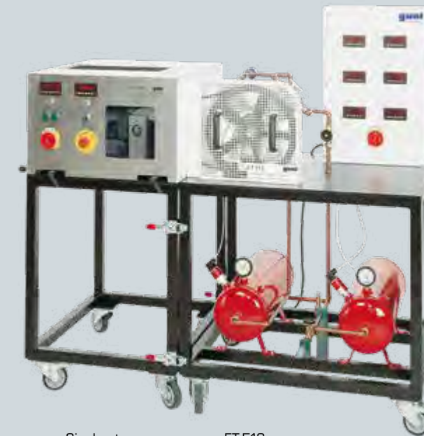
Single-stage compressor ET 513 with drive unit HM 365
