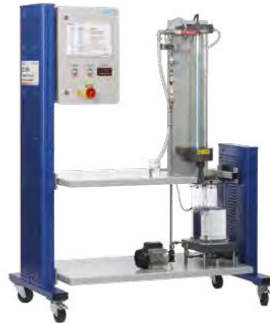
CE 584 Advanced oxidation Oxidation of organic substances with hydrogen peroxide and UV light
