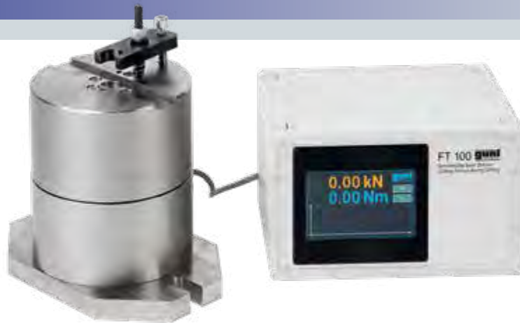
FT 200 Forming by bending Vice experiment: permanent deformation of flat bars
