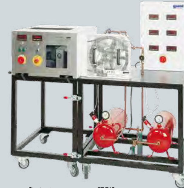
Single-stage compressor ET 513 with drive unit HM 365
