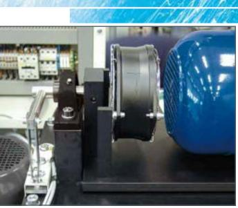
A force sensor detects the torque at the generator's
