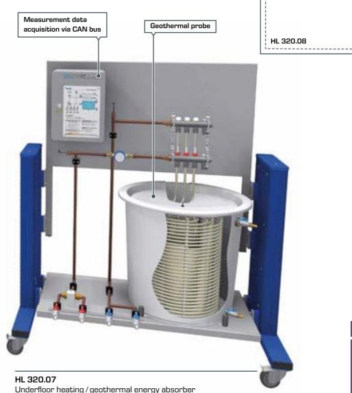
Underfloor heating / geothermal energy absorber
