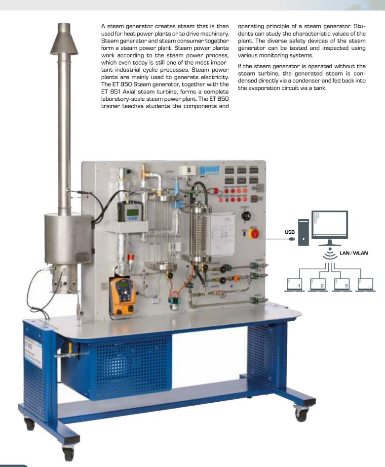
The steam generator is designed and pressure tested according to the "Technical Regulations for Steam" (TRD, Technischen Regeln Dampf) and has all safety valves prescribed by law.
