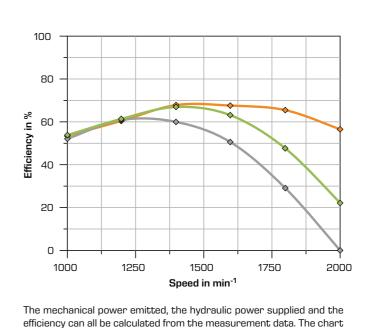
efficiency can all be calculated from the measurement data. The chart shows how the efficiency depends on the speed for three different distributor positions.
