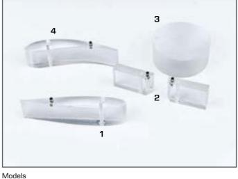
1 aerofoil, 2 orifice plate, 3 cylinder, 4 guide vane profile
