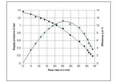
In the case shown here, the energy balance results in maximum efficiency at a flow rate of 25 L/min
