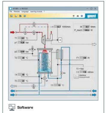
Sensors record temperatures, pressures and flow rates at all relevant points. Turbine speed and torque are measured electronically at the eddy current brake. The measured values are read from digital displays and can be transmitted simultaneously via USB directly to a PC where they can be analysed using the software included.
