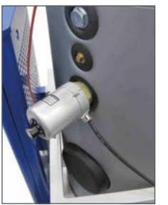
The storage tank is emptied in preparation for the experiment. Subsequently, the auxiliary heater can easily be inserted in just a few steps.
