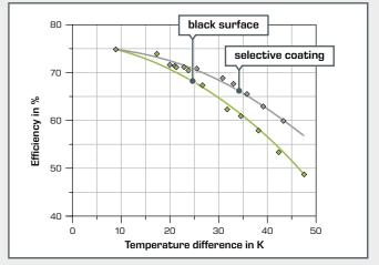
Efficiency depending on the collector temperature. A special coating of the absorber allows higher efficiencies.
