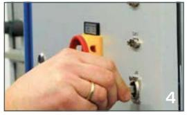
Secured cable connections (1, 2) allow safe modification of the cable routing. Current system data can be visualised both on the controller (3) and via a network connection (4).
