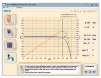
In simulation mode, it is possible to study the effects of specific cell parameters on the current/voltage characteristic.
