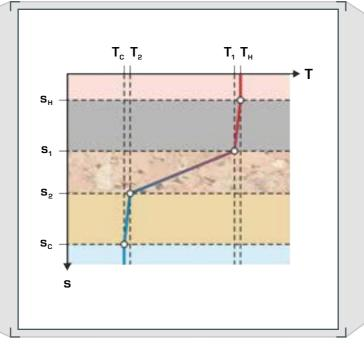
The analysis of the experimental data clearly shows the temperature gradients across the cork material. The hot plate, clamping plate and cold plate only show very small temperature gradients due to the much higher thermal conductivity of copper.
