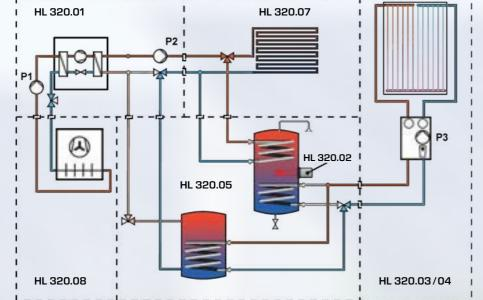
Example for a system schematic for complementary heating and domestic water heating with a solar thermal collector and a heat pump (combination 5).
