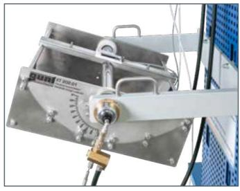
pivoting parabolic trough collector
