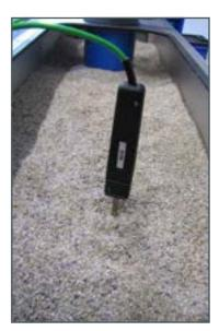
Temperature measurements with hand-held probe
