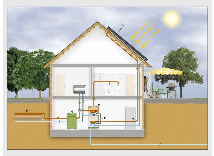
1 flat collector, 2 heat exchanger, 3 hot water storage tank, 4 heat pump, 5 geothermal energy absorber;
