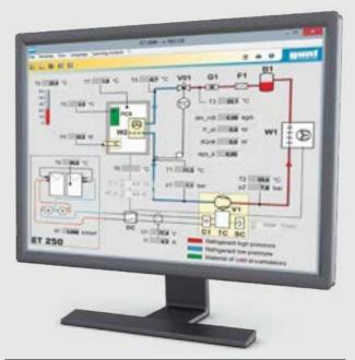
$\ensuremath{\mathsf{GUNT}}$  software for controlling the device and for measurement data acquisition via  $\ensuremath{\mathsf{PC}}$
