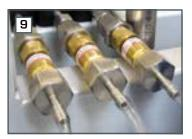
Connectors for biogas without gas analysis
