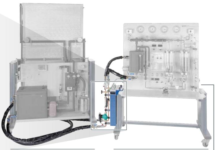
HL 313 Domestic water heating with flat collector or HL 314 Domestic water heating with tube collector
