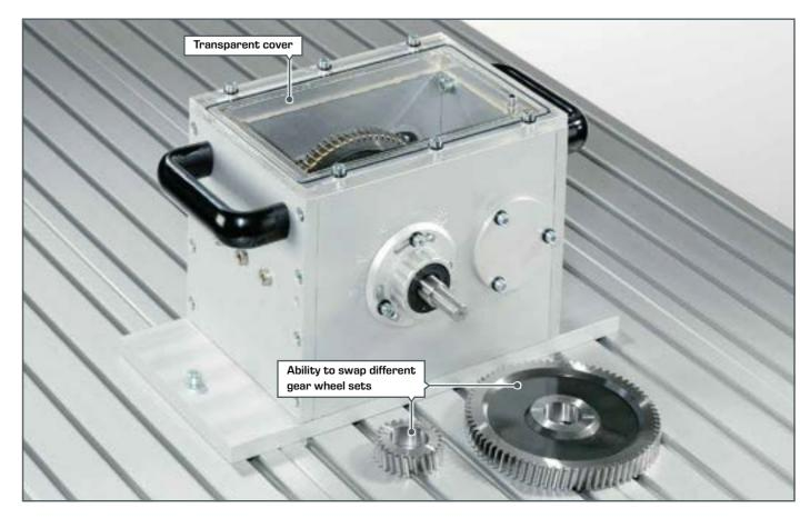
The PT 500.15 accessory set provides you with a variety of gear wheel sets with damaged teeth. Undamaged wheels are also included for comparative measurements. PT 500.15 enables of toothing damage and on locating damage in gears.
