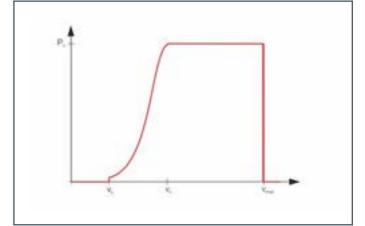
Power curve for autonomous mode with increasing wind velocity: power output is limited by the turbine control system by adjusting rotor speed and rotor blade angle
