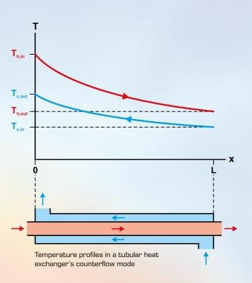
In counterflow mode, the cold medium exits at the input of the hot medium. If the heat exchanger is well designed, it is possible to achieve a higher outlet temperature on the cold side than on the hot side.
