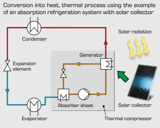
In solar refrigeration machines, the electric compressor is replaced by a thermal compressor.
