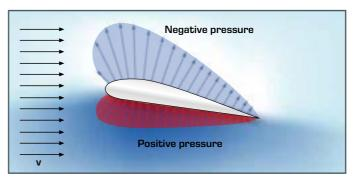
In order for lift to occur on a body under surrounding flow, there must be positive pressure on the underside of the body and negative pressure on the upper side.
