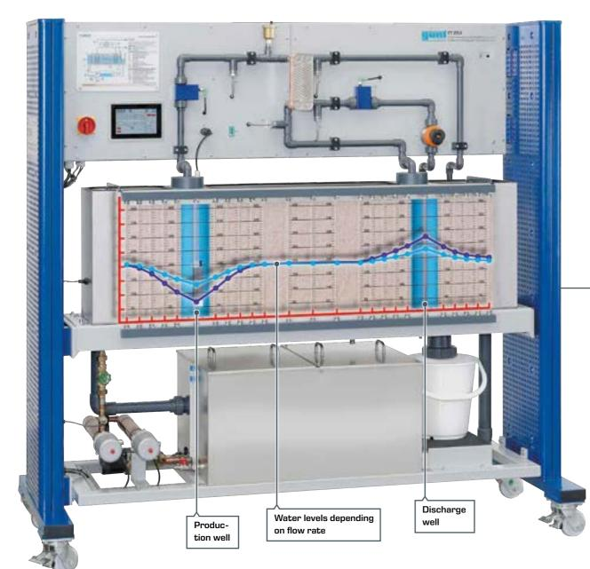
The core element of the trainer is a sand bed through which water flows, with a production well and a discharge well. The simulated groundwater flow can enter and exit the sand bed via two laterally adjacent chambers with adjustable fill levels. The water is supplied via a heatable water circuit with storage tank and pump.
