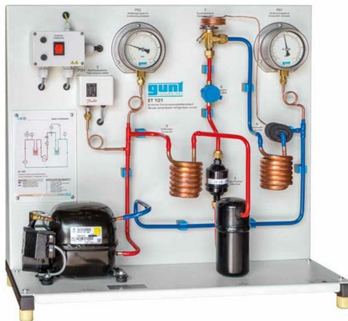
This experimental unit allows you to explain the structure and function of a heat pump using a simple compression refrigeration circuit, and tangibly demonstrate it for your students.
