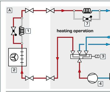
In heating mode the heat exchanger of the inner unit operates as a condenser
