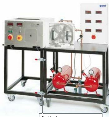
Combination: Setup of a complete compressor system together with the HM 365 universal brake and drive unit.
