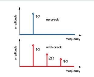
The opening and closing of a crack during one revolution of the damaged shaft leads to additional frequency components. The second order harmonic in particular increases rapidly compared to the undamaged shaft.
