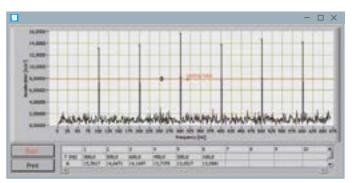
Spectrum of a straight-toothed gear at 1800min  $^{-1}$  and tooth engagement frequency of 752Hz
