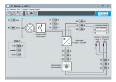
The generated electrical energy is transferred to the ET 220 control unit or the separate ET 220.10 control unit and can be used to charge the accumulators or for direct consumption.
