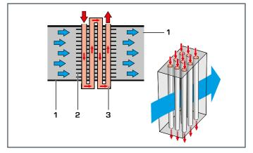
1 air duct, 2 fins, 3 water pipe section, cold air, pipe section with hot water
