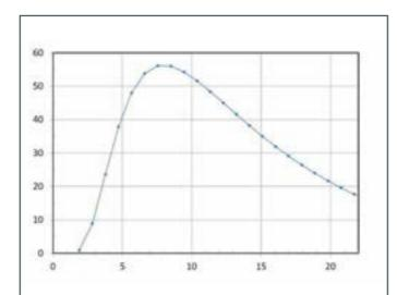
Simulated torque characteristic of a wind rotor: x axis: shaft speed in min- $^{1}$  y axis: torque in Nm
