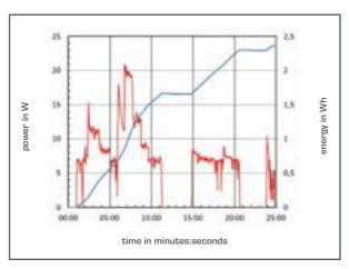
As a typical diagram from the ET220 manual shows, power curves (red) caused by the weather are analysed to calculate the energy yields (blue).
