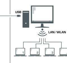
The measured values are displayed on the trainer and can simultaneously be transmitted via USB directly to a PC, where they can be analysed using the GUNT software included. The network-capable software makes it possible to follow and analyse the experiments at any number of workstations via a LAN/WLAN connection to the local network. The measured values are used to simulate a heat pump connected to the twowell system.
