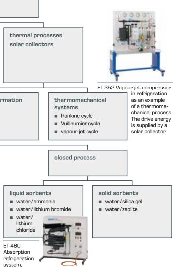
as an example of a closed process with the liquid sorbents water and ammonia.
