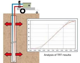
The second section of the trainer allows the study of the Thermal Response Test (TRT) used to evaluate the yield of a geothermal heat source.
