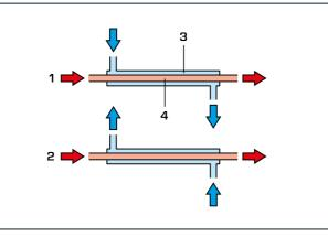
parallel flow operation, 2 counterflow operation,
