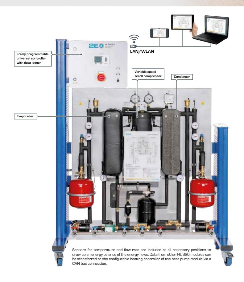
The HL 320.01 heat pump is part of the HL 320 modular system and provides you with a variety of combination options of geothermal and solar thermal energy in a modern heating system. The heat pump is driven by a variable speed scroll compressor. This means it is possible to adapt the heating power of the heat pump to the current demand of the heating system.
