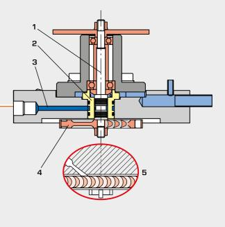
1 shaft, 2 labyrinth unit, 3 steam inlet, 4 rotor, 5 sectional view of nozzle and blades
