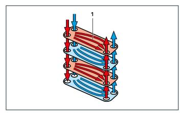
1 plate with pressed profilecold water side, hot water side
