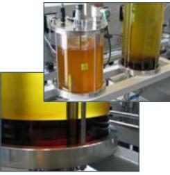
Transparent tanks allow continuous observation of reactions and separation processes
