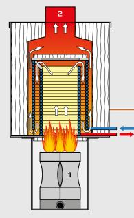
Sectional view of the ET 850 Steam generator 1 burner, 2 exhaust gas, 1 direction of flow of the heated air
