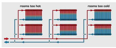
Temperature distribution in radiators without hydronic balancing
