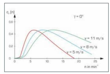
Power coefficient as a function of rotor speed: simulation of typical characteristic diagrams at different wind velocities and rotor blade angles
