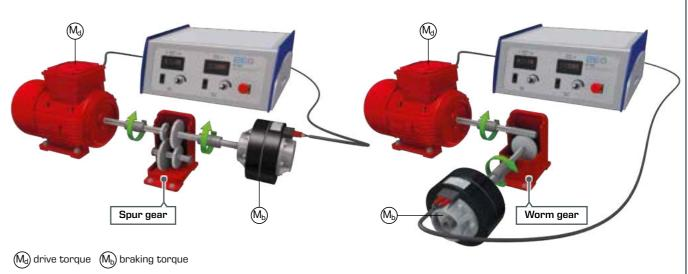
Energy losses in the gear mainly occur due to friction in the bearings and gear wheels. Friction converts kinetic energy into thermal energy. This energy is removed from the system and is therefore no longer available to produce electricity.
