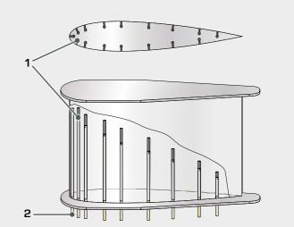
The blade profile has openings 1 for pressure measurement at regular distances on the upper side and the underside. Hoses 2 connect the blade profile to pressure sensors.
