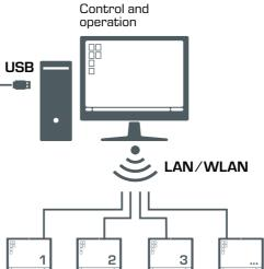
The software displays the measured values in a system diagram and enables the recording of individual measuring points or a time function. Stored measurement data can
