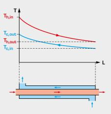
Temperature profiles in **counterflow operation** in a tubular heat exchanger
