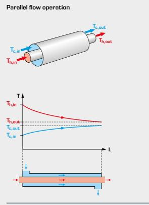
Temperature profiles in **parallel flow operation** in a tubular heat exchanger
