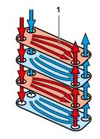
1 plate with pressed profile 🗖 cold water side, 📕 hot water side
