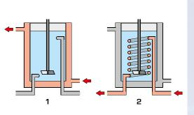
1 heating via the jacket, 2 heating via the coiled tube cold water side, hot water side
