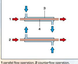
3 outer tube with cold water, 4 inner tube with hot water cold water side, hot water side
