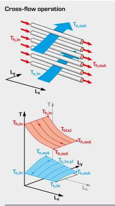
Temperature profile for a single row of tubes with single-sided mixed  $\ensuremath{\mathsf{cross\,flow}}$
