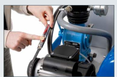
Checking the belt tension
