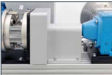
mechanical protection, input shaft/clutch, input side
