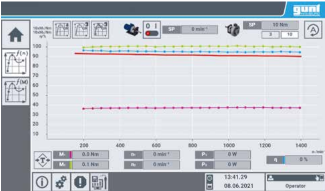
M = 10 Nm = constant, n = 200 - 1400 min -1 upper curves, red: efficiency curve setpoint
